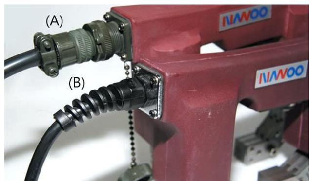
(A) Cable connector type (B) Intergrated Cable type
