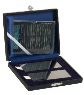
The Reference test block 1 acc. to EN ISO 3452-3 serves for the control of the sensitivity to indiation of liquid penetrants.
