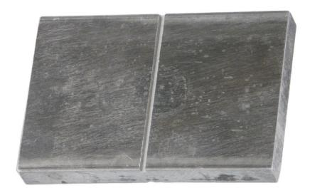
The ASTM test block is made of aluminum. It is divided into two areas (A and B) by a groove. It is intended for testing the display sensitivity of the testing equipment. In area A, the penetrant currently in use is applied, in area B the "fresh" penetrant is applied.
